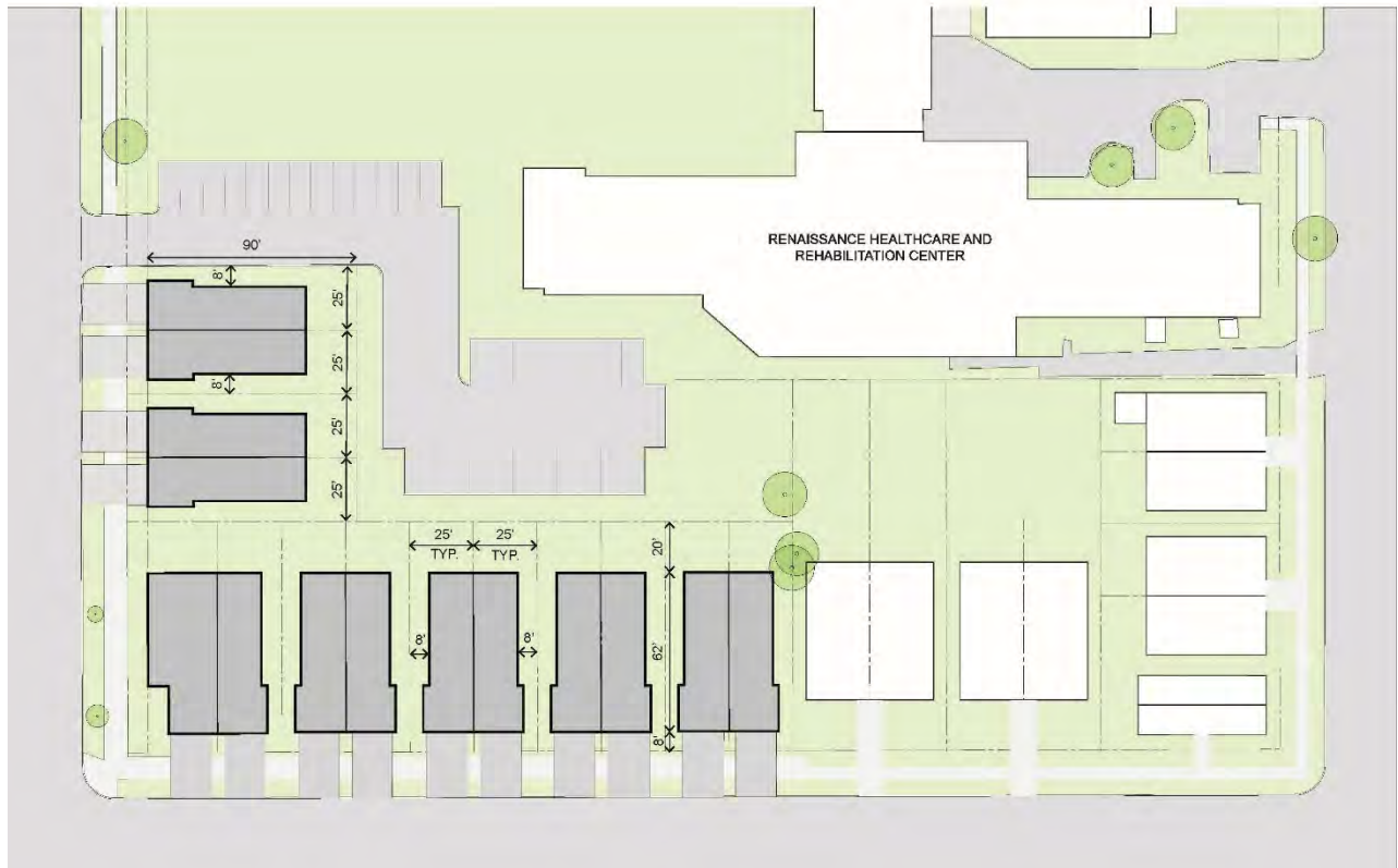
Parking illustration for by-rights development; curb cuts along Chester Avenue and 48 th Street with loss of street parking and green space.
